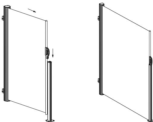
2. When you want to close it, to hold the handle and pull up the handle spindle. Keeping the fabric horizontal and push the handle back to the cover slowly.
