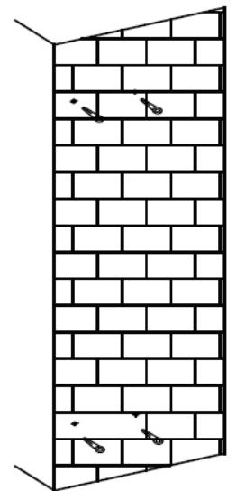
3. Fix the bracket with ST4.6×60mm cross tapping screw
